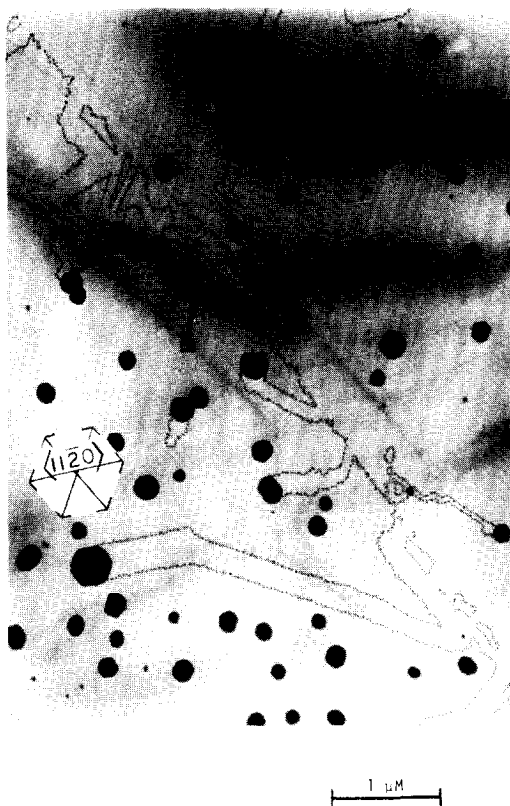
FIG. 1. Platinum particles channeling at 850°C in 1.0 atm hydrogen for 45.0 min. This shows a step in the basal plane to be a reactive site which initiates channels.
