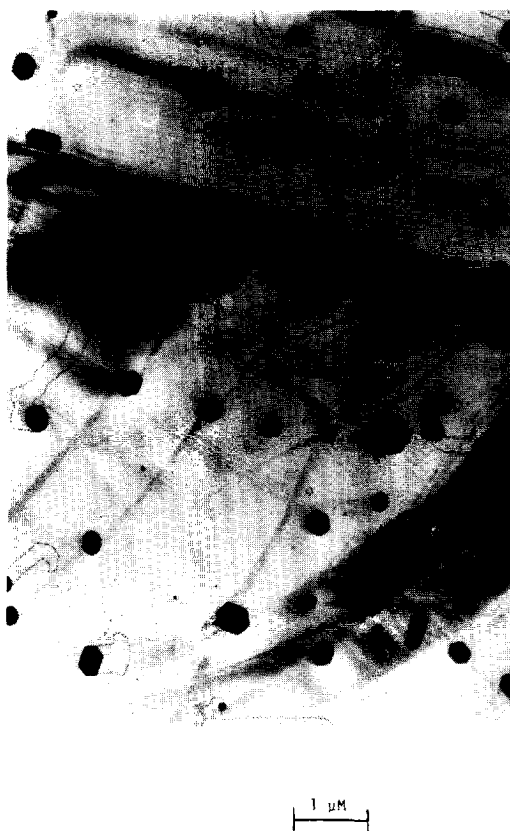
FIG. 3. Platinum particles reacted at 850°C in 1.0 atm hydrogen for 45.0 min. This shows vacancy-originated channels crossing paths and illustrates equal channeling depths.
